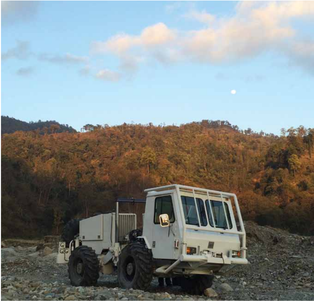
The Envirovibe minibuggy sends vibrations into the rock layers beneath the ground, gathering data that allows them to better visualise subsurface faults. The Ratu River Expedition, a documentary film produced by Isaac Kerlow, features the research of Hubbard and the tectonics group.
