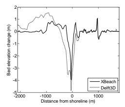
Fig. 12The bed elevation change simulated by XBeach compared to the results by Delft3D considered both hindered settling effect and stratification effect.
