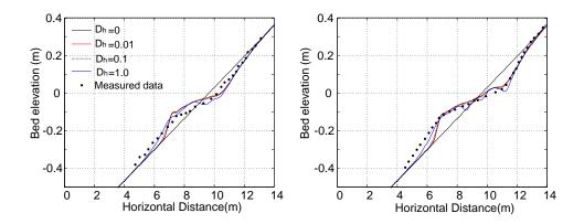
Fig. 14 Erosion and deposition after (a) 4 consecutive solitary waves and (b) 8 waves, with different horizontal diffusivities in XBeach
