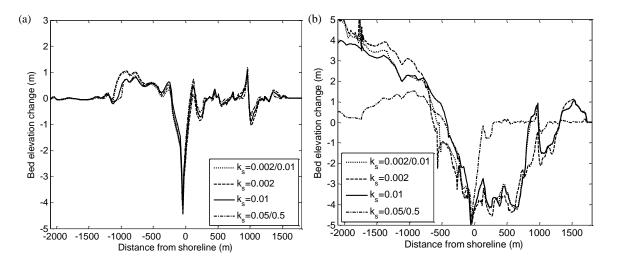
Fig. 13 Bed elevation changes with different bottom roughness (a) XBeach; (b) Delft3D
