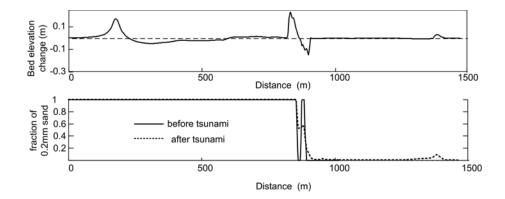
Fig. 16. Upper: bed elevation change for section E-E; Lower: the fraction of 0.2 mm sand along section E-E for S2. A value of 1 corresponds to 100% of fine sand (0.2mm), a value of 0.5 corresponds to 50% of fine sand and 50% of medium sand, a value of 0 corresponds to 100% of medium sand (0.4 mm).
