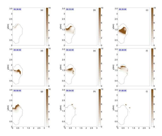
Fig. 14. Snapshots of suspended sediment concentration (kg/m<sup>3</sup>) during the first 1 hours. Concentration greater than 10kg/m<sup>3</sup> are not resolved.
