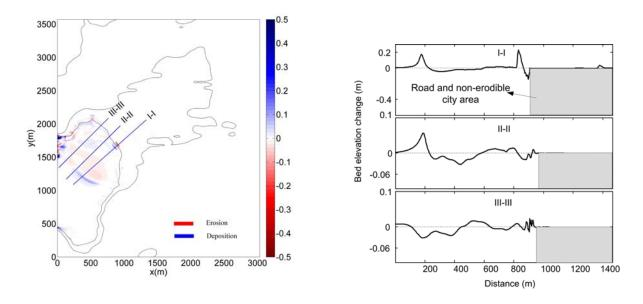
Fig. 15. Left: erosion and deposition map for S3; Right: bed elevation change for cross-sections I-I, II-II, III-III
