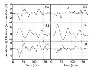
Fig. 4. The time series of the surface elevation (from COMCOT) at point P1 (shown in Fig. 1) on the open boundary
