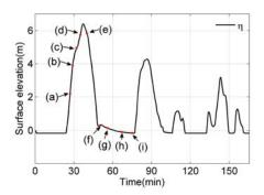
Fig. 9. Time series of velocity magnitude (left) and surface elevation (right) at point G1 (see Fig. 7). The labels (a)-(i) refer to the times at which the snapshots are taken of the concentration of the suspended sand in the flooding water.
