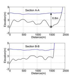
Fig. 7. Left: Map of the maximum inundation depth (m) in Painan city for Scenario S2; Right: water surface and topography in section A-A and section B-B.
