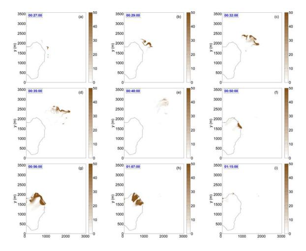
Fig. 10. Snapshots of suspended sediment concentration (kg/m<sup>3</sup>) during the first 1.5 hours. Concentration greater than 50kg/m<sup>3</sup> are not resolved.
